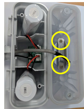
LED Head and Batteries LED screws highlighted
